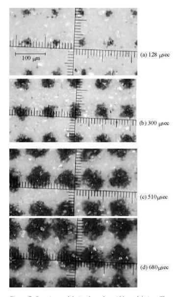
Figure 7. Dot size modulation by pulse width modulation. The recording frequency was 1 kHz.
