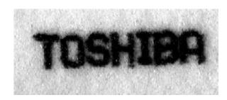
Figure 6. Micro structure letters with  $10 \times 14$  dots and a quarter millimeter square
